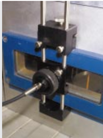
PCM 420 Directional Probe attached to chamber using the Universal Mount
